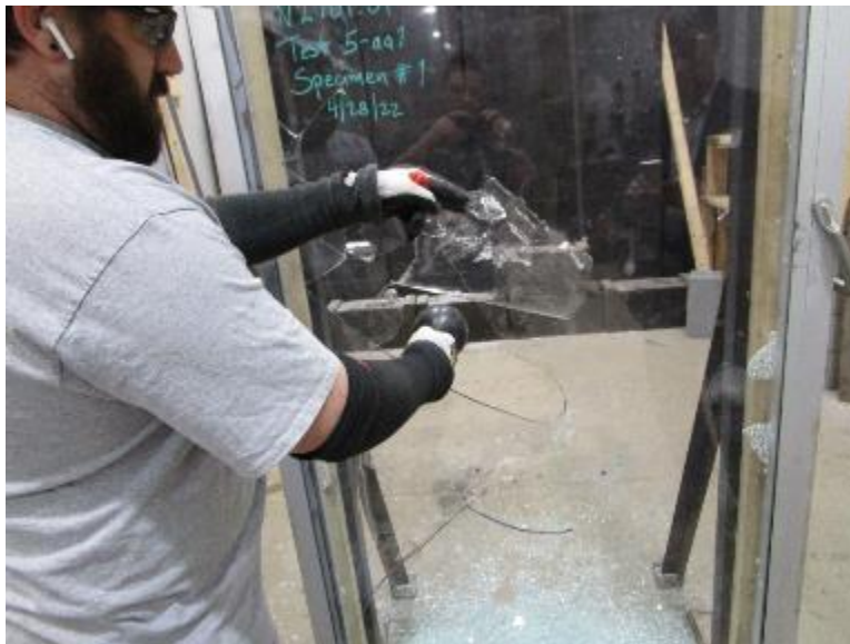
Photo No. 4 Forced Entry Resistance Testing Part 2, Failure - Post-Test Exterior
